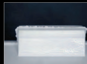
■ Welds on a molded item
