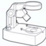
ABZ Rigid-arm w/tungsten 6V 7W trans/incident lights
