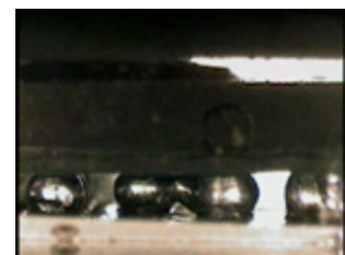
Bridge with Back Lighting
