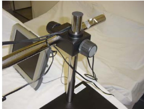
Assemble the Universal Stand as Shown
