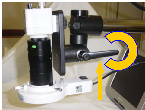
Use the knob to adjust viewing angle (Top down shown)
