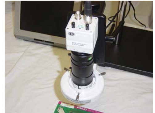
Attach the ring fluorescent light if desired
