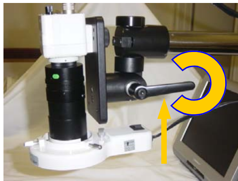
Use the knob to adjust viewing angle (Top down shown)
