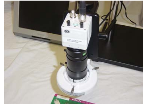
Attach the ring fluorescent light if desired
